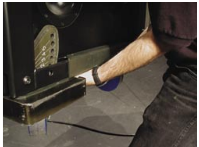
Figure 23. Removing caster rail
